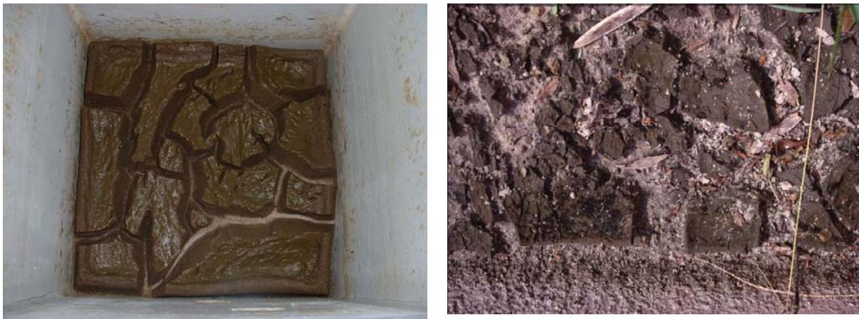
Figure 3. Alum Floc Drying Process.
